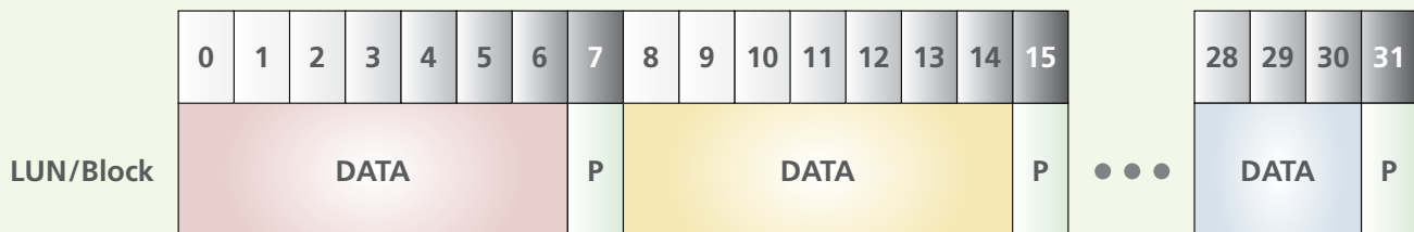
Figure 7: Fixed architecture per channel of the SSD to ensure proper data management
